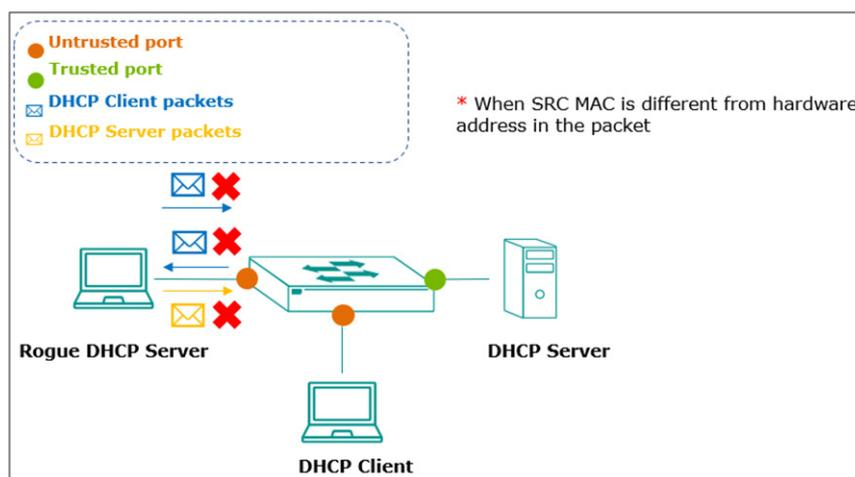
Successful DHCP transactions with DHCP snooping enabled will create and update the binding database. The binding database contains VLAN IDs, MAC addresses, untrusted ports of DHCP clients, and IP addresses. The binding database can also be used for other security functions such as IP Source Guard and Dynamic ARP Inspection.
