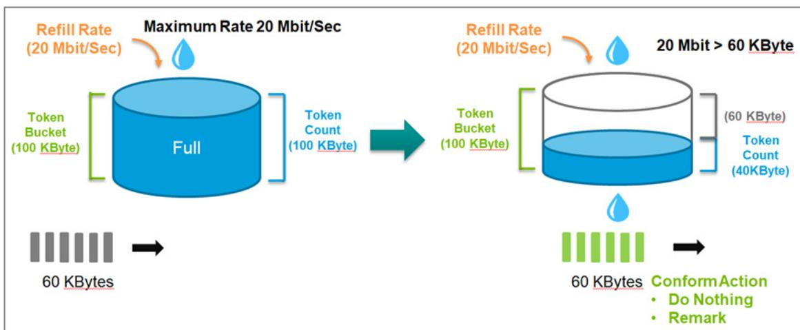
Token Bucket is an algorithm that is demonstrated as a container in the image below. The token can be seen as a marker to mark a packet that is allowed to be transmitted through this switch. When the token is flowing into the bucket, the length of the bucket
