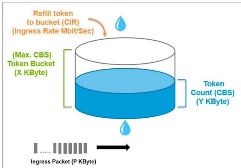
**CAR (Committed Access Rate)** is a traffic control mechanism used to ensure that packets meet the network rules before they enter the network. CAR can guarantee the traffic flow is under user-defined control; the packets exceeding the rule will be either dropped or remarked and transmitted again. When network traffic is jammed, these packets will be dropped first.
