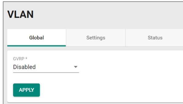
The screenshot shows the 'VLAN' configuration page with three tabs: 'Global', 'Settings', and 'Status'. The 'Global' tab is active. Underneath, there is a dropdown menu for 'GVRP \*' currently set to 'Disabled'. Below the dropdown is a green 'APPLY' button.
