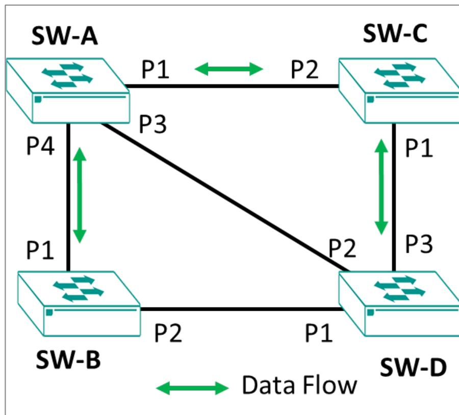
Ordinarily, data will flow from SW-A directly to SW-B and SW-C. SW-D data will transit SW-C. However, if something happens that breaks links, data flow can be rerouted without administrator intervention. Follow the subsequent examples to configure each switch.
