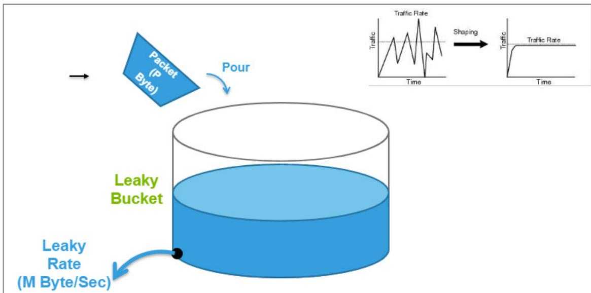
If incoming packets would exceed the capacity the bucket, those packets would be non-conforming, and are not added to the bucket (dropped). Data will be added to the bucket as space becomes available for conforming packets. To setup Egress Shaper on a specific port, you will need to provide CIR (Committed Information Rate) and CBS (Committed Burst Rate) values.
