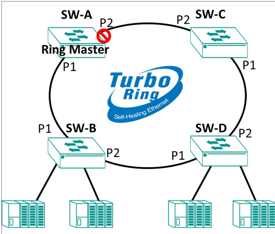
Set up Turbo Ring v2 to connect multiple networks of machines and devices to create a fault-tolerant network and achieve continuous operations.
