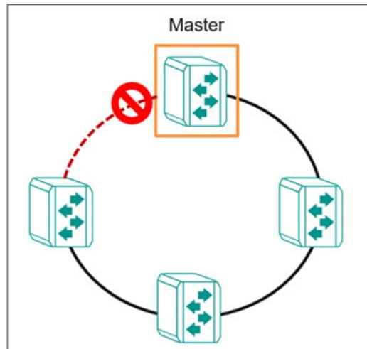
Turbo Ring v2 allows connected network devices to elect a "master" switch, which blocks packets from traveling through any of the network's redundant loops and manages the network. If a section breaks, the protocol adjusts the ring so that the disconnected parts of the network establish contact. This enables continuous network operations, even when there is a fault in the network.
