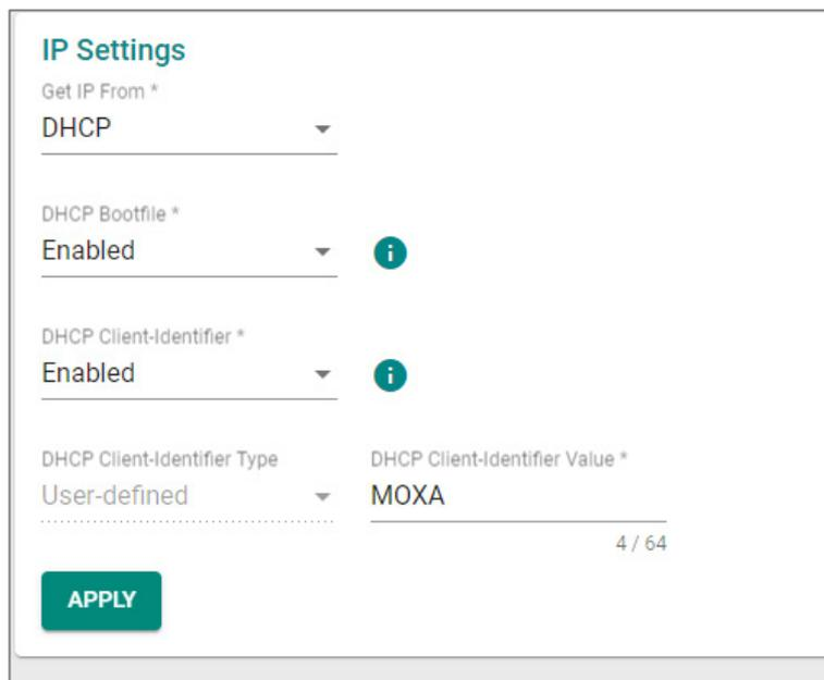
A screenshot of the 'IP Settings' configuration page. It includes several fields: 'Get IP From \*' set to 'DHCP', 'DHCP Bootfile \*' set to 'Enabled', and 'DHCP Client-Identifier \*' set to 'Enabled'. Below these are 'DHCP Client-Identifier Type' set to 'User-defined' and 'DHCP Client-Identifier Value \*' set to 'MOXA'. A green 'APPLY' button is at the bottom left. A page number '4 / 64' is visible at the bottom right.
