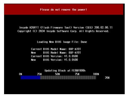
When the upgrade is finished, the computer will automatically reboot.
