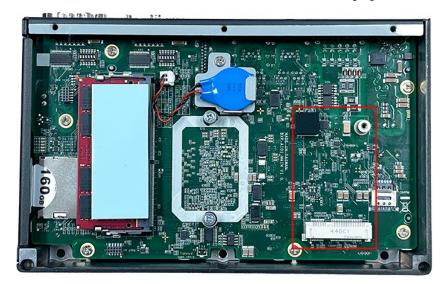
3. Install the Mini PCIe module in the socket.
