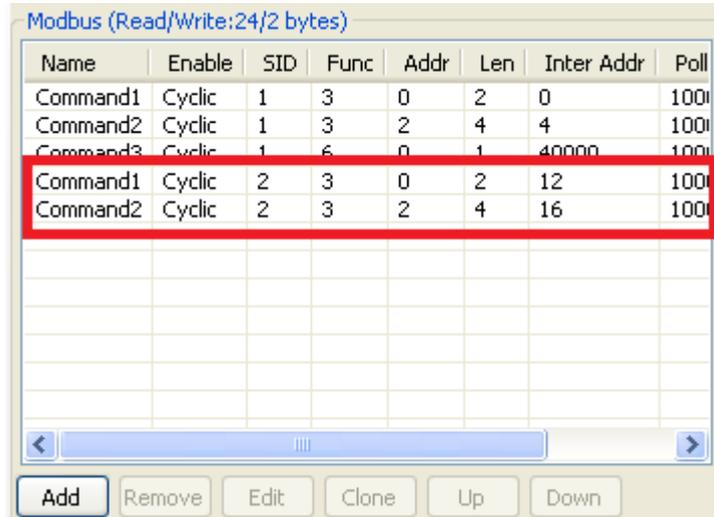
After all Modbus requests finish, all the data collected from Modbus should be mapped to PROFIBUS I/O modules for the PROFIBUS Master to use.
