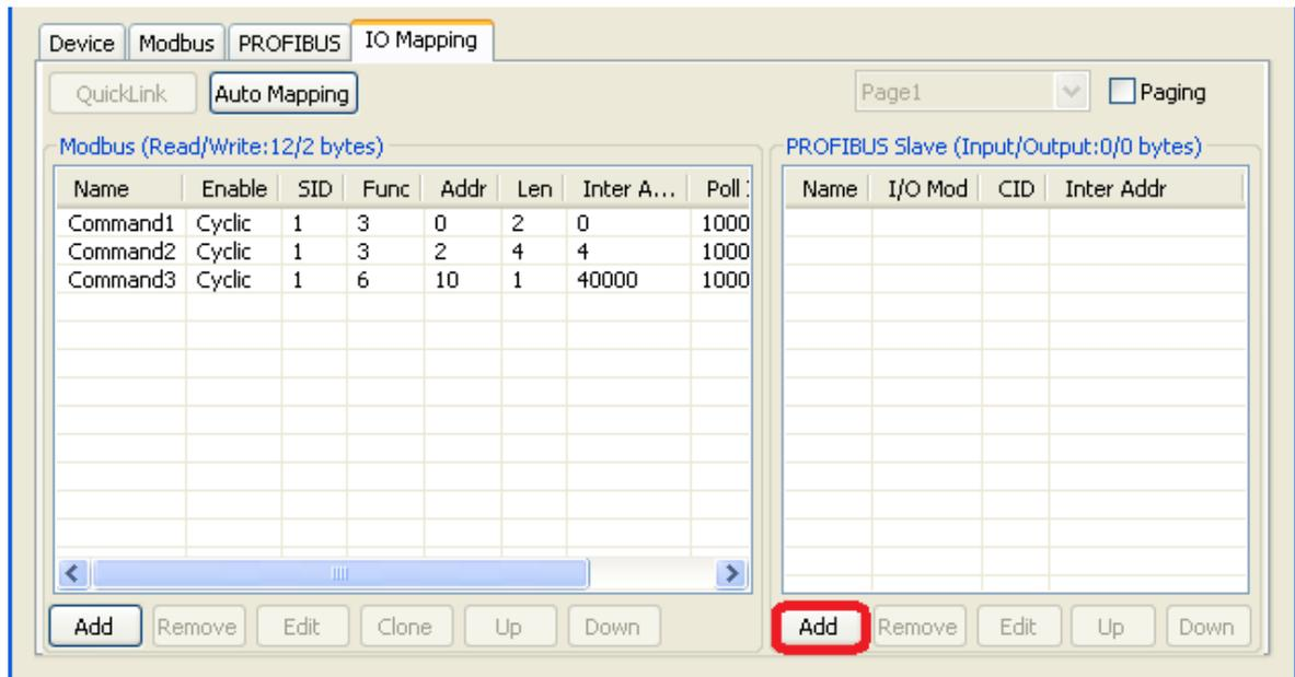
Then, a dialog which is used to set up the IO module will appear. Please adjust the parameters that correspond with the Modbus requests you set before. Click **OK** to record this IO module.
