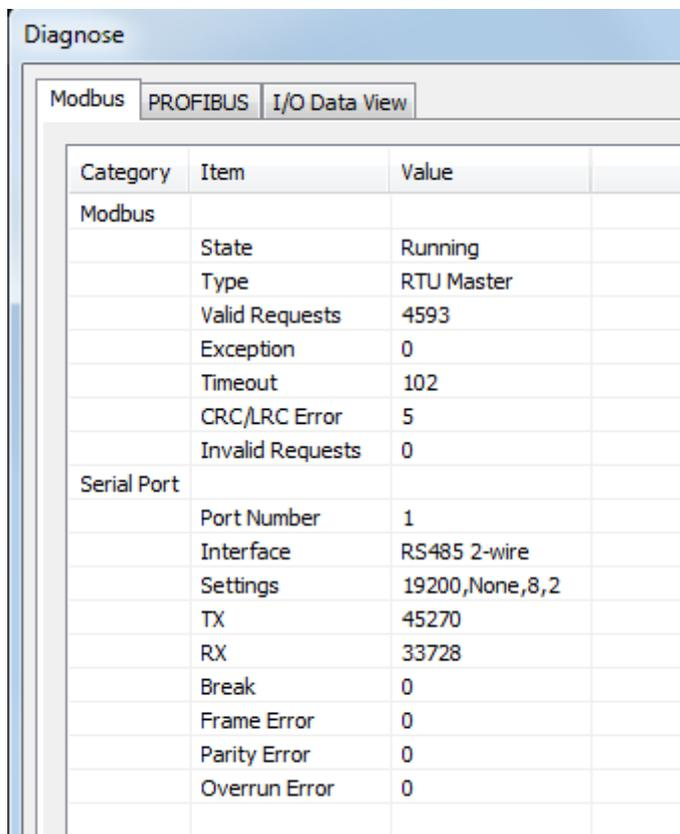
There are two parts. In Modbus tab, the first part is the information regarding Modbus. These details will help you analyze the Modbus communication.
