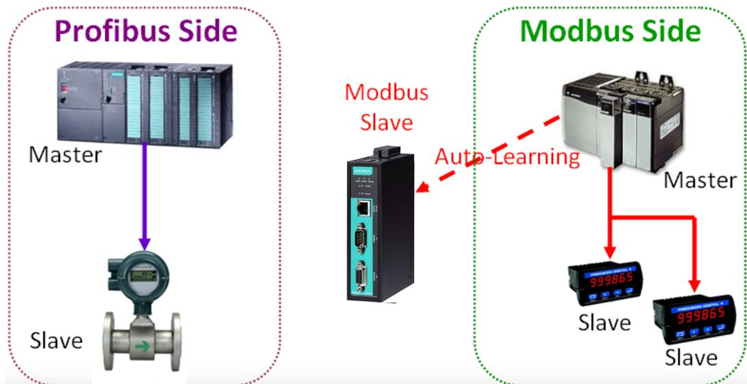
After some time, MGate 4101-MB-PBS will fully learn the requests from the Modbus client/master. Through this QuickLink process, the MGate 4101-MB-PBS can replace the legacy Modbus client/master. Moreover, the MGate 4101-MB-PBS can respond to all the Modbus servers/slaves correctly.
