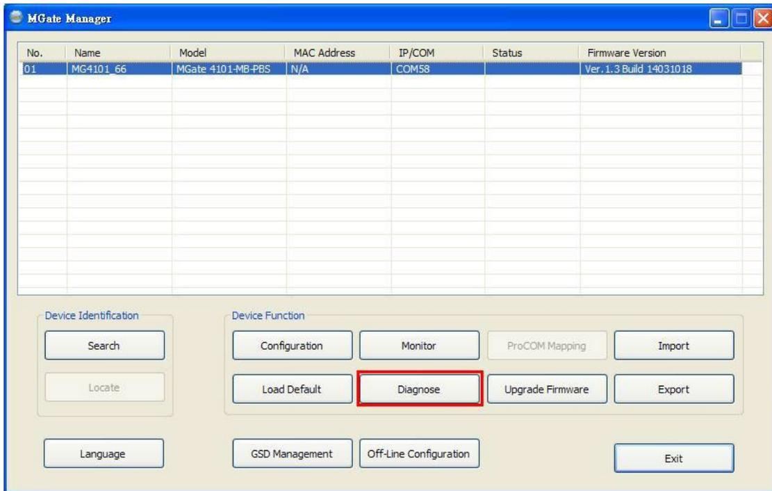
The dialog box will show the details of the communication status of Modbus, PROFIBUS, and I/O Data View. In addition, it contains serial parameters.
