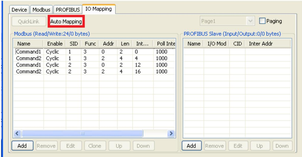
Click the **Auto Mapping** function. Then, a dialog box that is used to select the package types will appear. Please select one of them to map Modbus commands. Click **OK** to produce PROFIBUS I/O modules.
