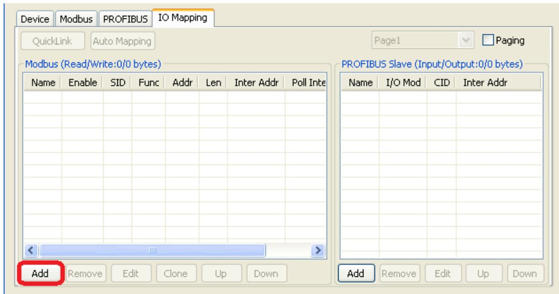
Each Modbus request includes Name, Enable, Modbus slave ID, Function Code, Address, Length, Internal Address, Poll Interval, Swap, Fault Protection, Fault Timeout. Please refer to datasheets or manuals of Modbus server/slave devices to fill out these fields.
