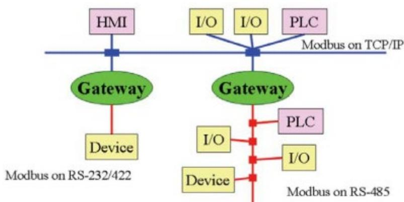
Ordinarily, Modbus TCP and Modbus ASCII/RTU cannot communicate with each other.
