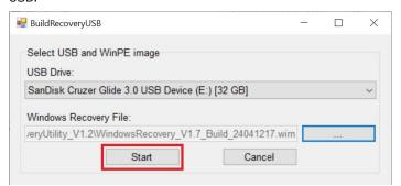
6. Wait for the process to finish. The program will format the USB device and create a UEFI bootable volume and a WinPE volume. You may see additional windows about folder information; do not close these. You can close the windows after the process finishes.
