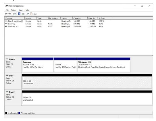
2. Right-click the target disk. Select the target volume type. For example: RAID1(Mirror).
