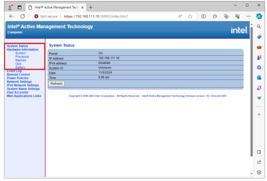
4. The Intel® AMT website provides the basic remote power control feature for the managed device. The advanced remote power control and the remote KVM feature please reference to next chapter.
