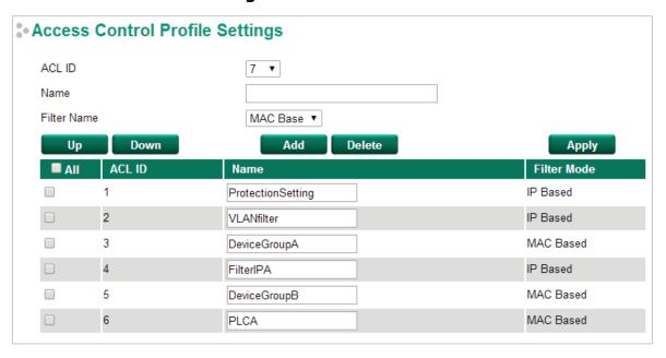
On this page, you can configure two settings: (1) Add/Modify Access Control list, and (2) Adjust ACL ID.
