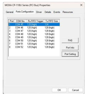
Select a COM number for the port from the **Port Number** drop-down menu. Select the **Auto** Enumerating COM Number option to map subsequent ports automatically. The port numbers will be assigned in sequence. For example, if COM 1 is assigned to Port 1, then COM 2 (if not already occupied) will be assigned to Port 2, etc.
