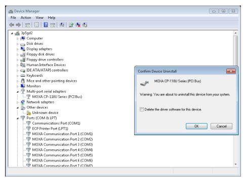
Select Delete the driver software for this device and click OK to proceed with uninstalling the board.
