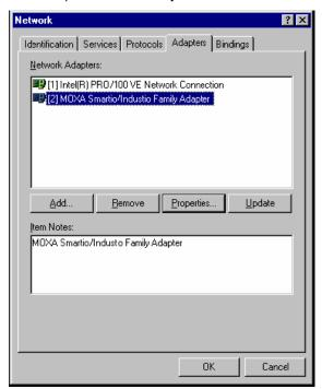
2. The configuration panel will open with a list of installed boards. Select your board and click **Property**. Up to four Moxa UPCI boards can be installed at a time.
