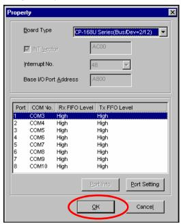
5. The board will now appear in the configuration panel (**CP-168U Series in this example**). Click **OK** to return to the Network applet. After that, click **OK** again to exit the Network applet
