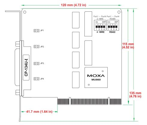
Onboard termination resistors can be activated individually for each serial port using jumpers JP1 through JP4. For CP-134U, JP1/2/3/4 corresponds to serial port 1/2/3/4, respectively. For CP-134U-I, JP1/2/3/4 corresponds to serial port 4/3/2/1, respectively. Short the jumper pins to activate the termination resistor; leave the jumper pins open to bypass the termination resistor.
