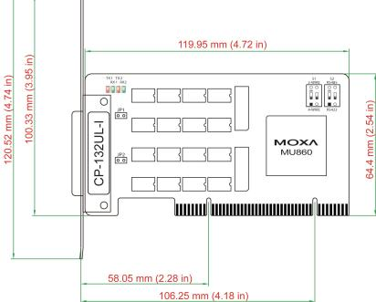
Onboard termination resistors can be activated individually for each serial port using jumpers JP1 and JP2. JP1 corresponds to serial port 1. Short the jumper pins to activate the termination resistor; leave the jumper pins open to bypass the termination resistor.
