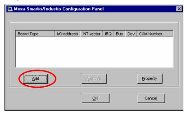
4. Under **Board Type**, select the UPCI board that is being installed. The window will show the COM settings for the serial ports on the board. Modify the COM settings for any port at this time by selecting a port and clicking **Port Setting**. If you are satisfied with the COM settings, click **OK** to return to the configuration panel.
