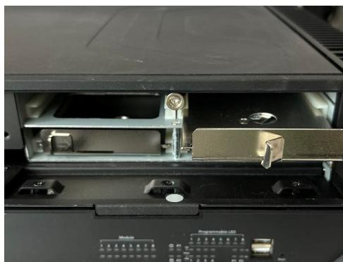
3. **Remove the expansion module slot door** (Moxa proprietary slot) by unfastening two screws.
