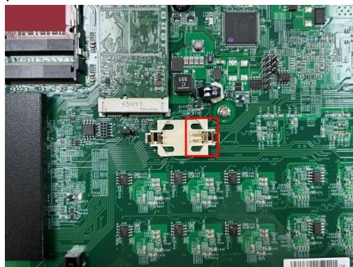
4. **Insert a new RTC battery.**
