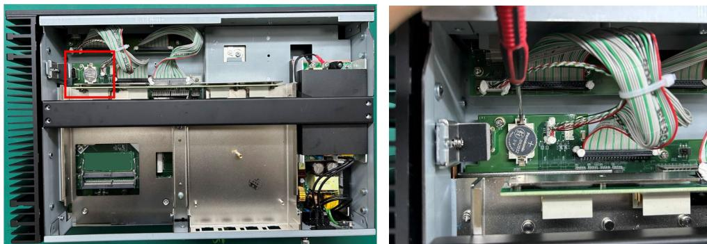
**Note** The battery holder without the battery is shown here. To easily release the battery, gently press the area marked with a flat-head screwdriver.
