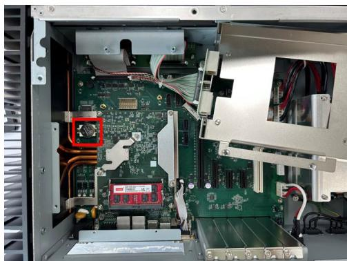
**Note** We recommend using a short screwdriver or screwdriver head to make it easier to reach and press the battery holder at a proper angle to release the battery. Gently press the area indicated in the figure.
