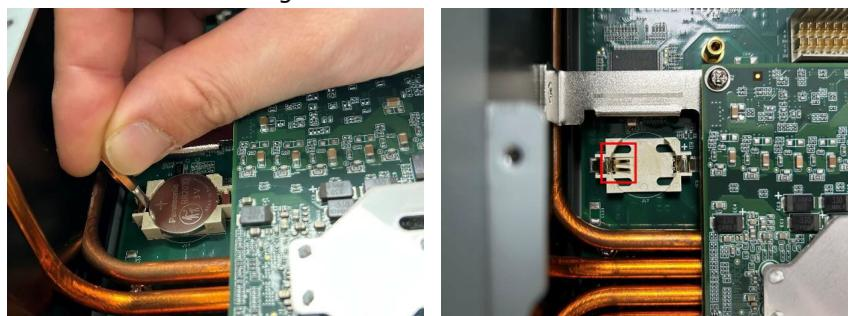
10. Insert a new RTC battery.
