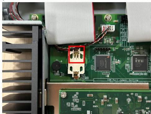
4. **Insert a new RTC battery.**
