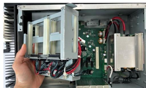
8. Remove the **Moxa proprietary slot case** by unfastening four screws (indicated in the figure) and lift it vertically to remove it.
