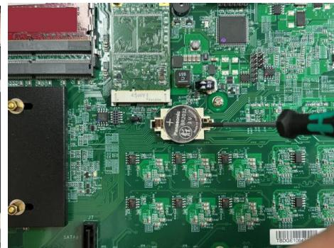
**Note** The battery holder without the battery is shown here. To easily release the battery, gently press the area marked with a flat-head screwdriver.
