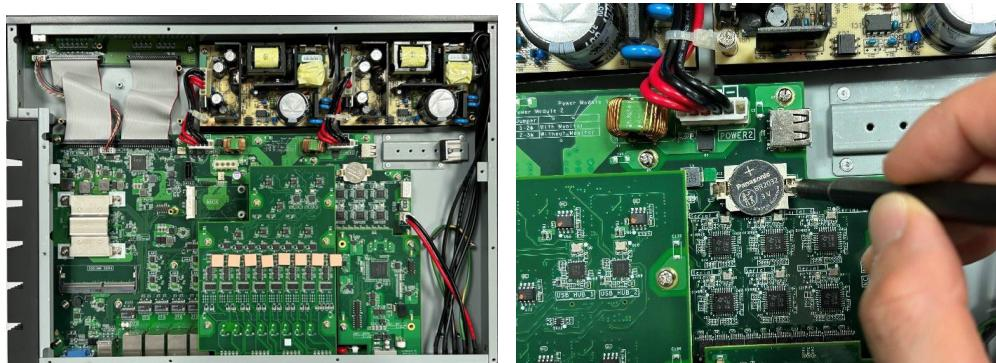
**Note** The battery holder without the battery is shown here. To easily release the battery, gently press the area marked with a flat-head screwdriver.
