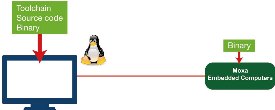
Moxa Industrial Linux (MIL) in Moxa's Arm-based computers is based on Debian. So, we recommend setting up a Debian environment on the host device to ensure best compatibility during cross compilation.
