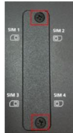
2. Insert a card in the SIM 1 slot. Make sure you insert the card in the right direction as indicated in the image beside the slot. (The notch on the SIM card should face outward.)
