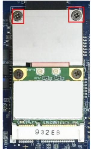
5. Attach one end of the Wi-Fi antenna cable to the connector on the Wi-Fi module and insert the other end (with the threaded connection ring) through the antenna mounting hole on the front panel of the computer.
