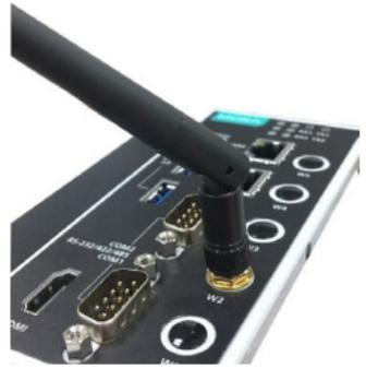
The pre-built cellular module comes with three SMA connectors for a GPS antenna (W4), a primary cellular antenna (W3), and a secondary cellular antenna (W1).
