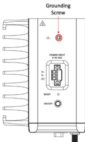
**NOTE** A 4 mm<sup>2</sup> conductor must be used when utilizing the connection to the external grounding screw. The heat sink is grounded to the chassis by an internal screw.
