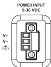
Use an Listed Power Supply (LPS, 9 to 36 VDC) or Class 2 power cord to connect to the AIG-502's terminal block to power jack converter and then turn on the power. The Power LED will light up to indicate that the power is supplied properly. The OS is ready when the Power LED glows a solid green.
