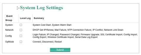
• To view events in the system log, log in to the HTTP/HTTPS console and select **System Monitoring > System status > System Log**.
