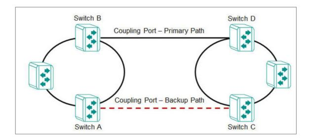
Ring coupling uses extra ports on each pair of coupled switches. In this example, that means:
