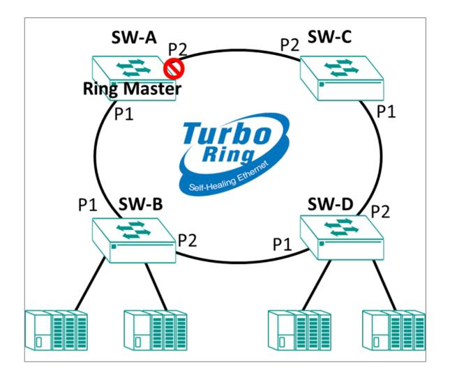
Set up Turbo Ring v2 to connect multiple networks of machines and devices to create a fault-tolerant network and achieve continuous operations.
