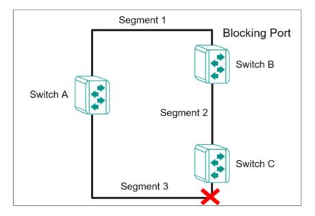
STP will determine which path between each segment is most efficient, and then assign a specific reference point on the network. When the most efficient path has been identified, the other paths are blocked. In the previous three figures, STP first determined that the path through switch C was the most efficient, and as a result, blocked the path through switch B. After the failure of switch C, STP re-evaluated the situation and opened the path through switch B.
