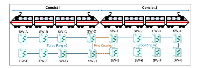
This structure allows for easy administration as consists are coupled and uncoupled.
