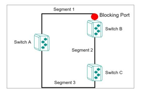
What happens if a link failure is detected? As shown in the figure below, the STP will change the blocking state to a forwarding state so that traffic from segment 2 flows through switch B to segment 1 through a redundant path.
