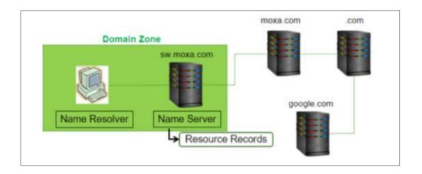
A domain name identifies a node. Each node has a set of resource information, which may be empty. The set of resource information associated with a particular name is composed of separate RRs. The order of RRs in a set is not significant, and need not be preserved by name servers, resolvers, or other parts of the DNS. The basic RR formats are defined in RFC 1034.
