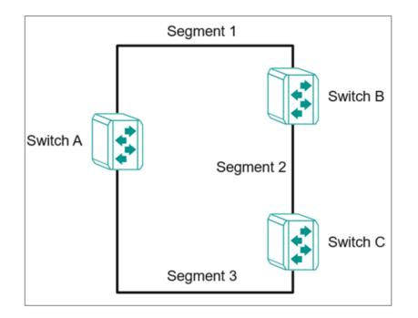
If STP is enabled, it will detect duplicate paths or block one of the paths from forwarding traffic. In the following example, STP determined that traffic from segment 2 to segment 1 flows through switches C and A since this path is in a forwarding state and is processing BPDUs. However, switch B on segment 1 is in a blocking state.
