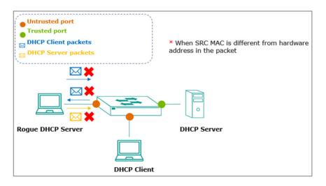
Successful DHCP transactions with DHCP snooping enabled will create and update the binding database. The binding database contains VLAN IDs, MAC addresses, untrusted ports of DHCP clients, and IP addresses. The binding database can also be used for other security functions such as IP Source Guard and Dynamic ARP Inspection.
