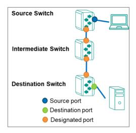
Ingress, egress, or both ingress and egress traffic of the source port(s) can be mirrored to one or more destination ports on destination switches.
