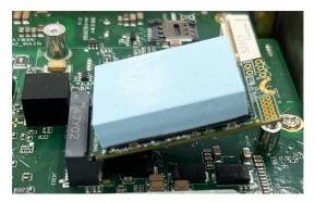
4. Fasten the screw to secure the module to the socket.
