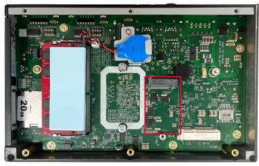
3. Install the M.2 module in the socket.
