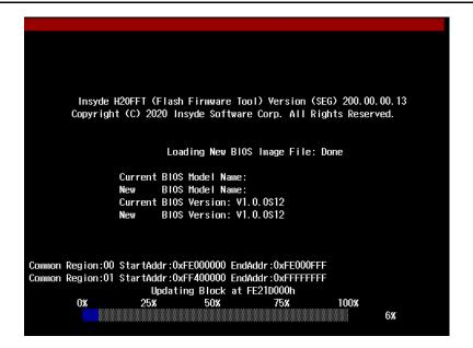
5. When the upgrade is done, the computer will automatically reboot. You can check the BIOS version on the Main page.
