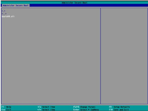
Enter "Administer Secure Boot" once again and see "Select a UEFI file as trusted for execution", put loader into the database named and followed by the UEFI standard \EFI\BOOT\BOOT\machine type short-name\}. E.g., efi\boot\BootX64.efi, Debian (EFI\debian\grubx64.efi), Suse (EFI\opensuse\grubx64.efi)
