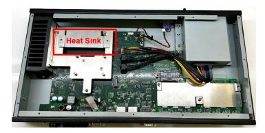
4. Unfasten the two M3x6 mm screws on the heat sink and remove the heat sink to reveal the memory slot.
