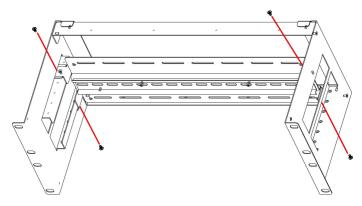
**Step 4:** Attach RK-4U into a 19"-rack cabinet and then mount the device onto RK-4U.
