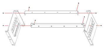
Step 2: Fix din rail one to the panel.
