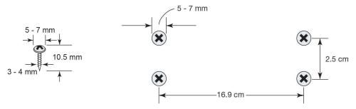
The head of the screws should be 5 to 7 mm in diameter, the shaft should be 3 to 4 mm in diameter, and the length of the screws should be at least 10.5 mm. Leave about 5 mm of space between the head and the wall.
