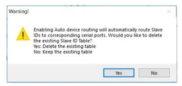
Click **Yes** to delete the existing (factory default or user-set) routing table; the auto-routing mechanism will automatically find the correct serial port that connects the target Modbus device. Moreover, if a device is added to the gateway later, the gateway can also route it correctly. Note that the routing table will be cleared as the warning message. The Slave ID table is then shown as in the figure below.
