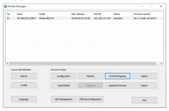
On the ProCOM mapping dialog box, you can map up to four ProCOM functions for each Modbus gateway to your PC's COM ports. The driver will generate virtual COM ports on your PC to connect to the selected MGate MB3x70 over the network.
