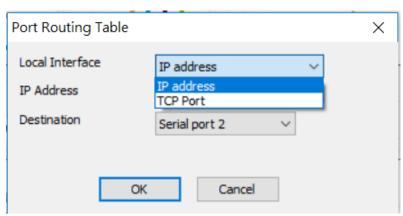
For example, you could assign TCP ports 2001 to 2004 to serial ports 1 to 4, respectively. When the gateway receives a Modbus request designated for TCP port 2001, it will forward the Modbus request to serial port 1 directly. Similarly, if it receives a Modbus request designated for TCP port 2004, it will forward the Modbus request to the serial port 4 directly.
