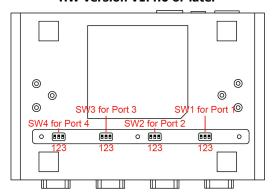
To access these switches, loosen the screws on both sides of the device and open the cover.
