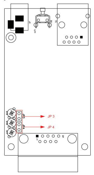
To access these jumpers, loosen the screws on both sides of the device and open the cover.
