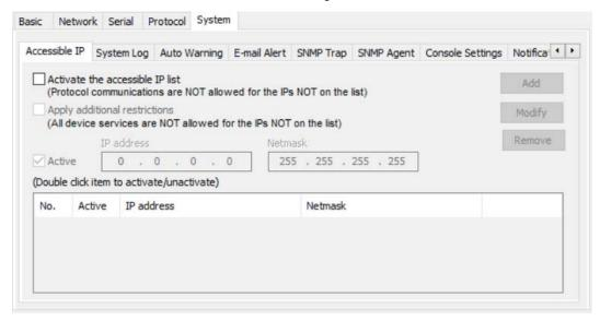
The Accessible IP List function allows you to add or block remote host IP addresses to prevent unauthorized access. Access to the MGate MB3000 is controlled by IP address. That is, if a host's IP address is in the accessible IP table, then the host will be allowed to access the MGate MB3000. The different restrictions are listed in the table below. The checkbox "Apply additional restrictions" can only be activated if the checkbox "Activate the accessible IP list" is activated.
