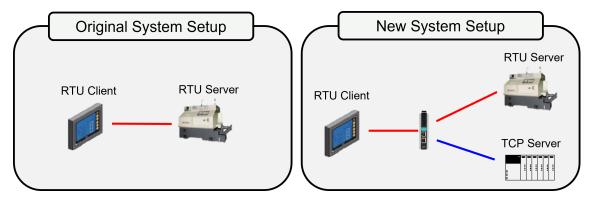
Under **Mode** settings, use the radio button to set up the operation mode for each serial port. If the Modbus RTU server/slave is connected to serial port 1, select "RTU Slave Mode" under port 1. If a Modbus RTU client/master is connected to serial port 2, select "RTU Master Mode" under port 2.
