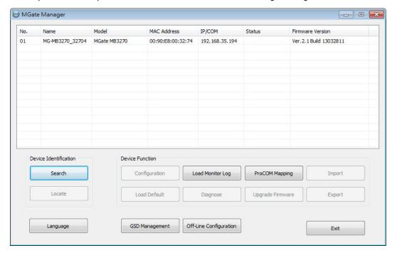
The second way is to right-click the item to begin the web console configuration. You must provide the correct password to log in to the web console.
