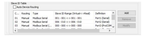
Select the second channel and click **Modify**. Since the virtual ID recognized by the Modbus client/master is 2, and the real slave ID of the device B is ID 1, the offset should be set as -1.
