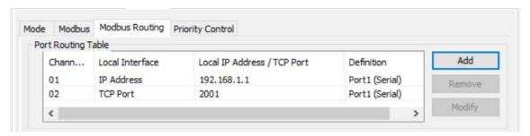
With port routing mechanisms, Modbus slave ID routing can be simpler and more effective by giving users the flexibility to define a multirouting mechanism.
