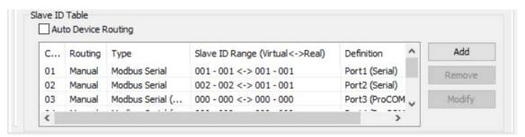
Now, the Modbus client/master can send a request with slave ID 1 to Modbus device A connected to serial port 1 as well as send a request with slave ID 2 to the Modbus device B connected in serial port 2.
