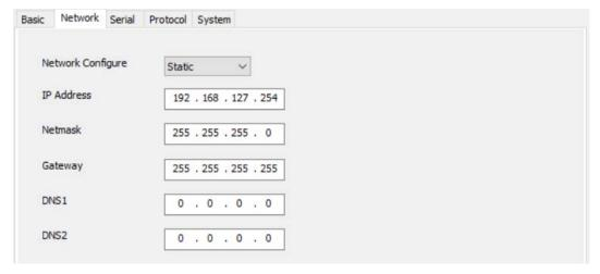
You can also change it on the web console. Click **Basic Settings > Network**. You can change the Name, IP Configuration, IP Address, Netmask, Default Gateway, and DNS. Click **Submit** to continue.
