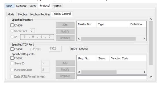
Priority control is designed for requests that are sent to Modbus RTU/ASCII servers/slaves. Since Modbus RTU/ASCII servers/slaves cannot handle multiple requests, the Modbus gateway must send each request individually and wait for the response before sending the next request. As requests stack up, the response time can suffer. This can cause problems for certain critical requests that require an immediate response.
