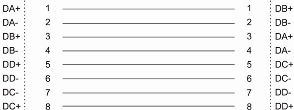
Straight-through Cable Wiring (MDI to MDI-X)
