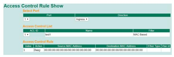
**NOTE** For TN-5800A series, there are two limitations on ACL settings. Based on the ingress port type of ACL rules, there are two types for the limitation of numbers.
