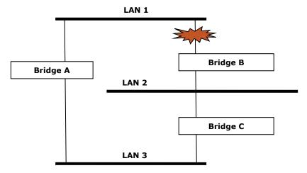
What happens if a link failure is detected? As shown in the next figure, the STP process reconfigures the network so that traffic from LAN segment 2 flows through bridge B.
