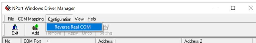
This is the TCP port number assignment for the remote host/server. It is the port number that the serial port of the NPort 6000 uses to establish the connections with Remote Host/Server. To avoid conflicts with well-known TCP ports, the default is set to 60950. Configure the mapped COM port.
