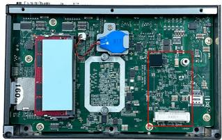
4. Install the Mini PCIe module in the socket.
