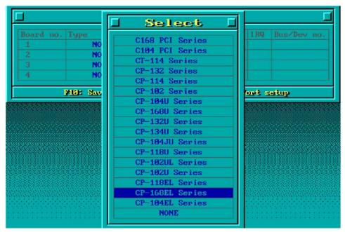
3. A window will open displaying basic configuration information for all boards of this type currently installed in the system. Press **PgDn** to configure the port settings.
