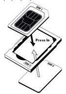
Insert the tray back into the slot.You will hear a click indicating the tray is locked into place.
