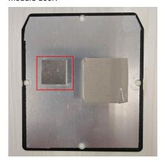
10. Take out the **Thicker thermal pad**. It has two protective films: one blue and one clear. The clear film covers the adhesive side, which should be attached to the aluminum block. Once attached, remove the blue film to expose the top surface.
