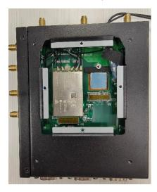
5. Take out the one of the thermal pad. It has two protective films: one blue and one clear. The clear film covers the adhesive side, which should be attached to the aluminum block.
