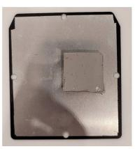
10. Reinsert the wireless module door and fasten it securely using the 4 Torx screws (6-point star ★).
