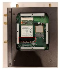
8. Take out the thicker alumin block, peel off the blue protective film to expose the adhesive side of the aluminum block, align it with the marked area (red box) on back of the wireless module door and firmly press it into place. The adhesive side should face downward to attach the block securely to the module door.
