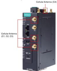
In addition, a GPS antenna connector is provided for the GPS module. All cellular and GPS connectors are of type SMA female. UC-4434, UC-4430, UC-4454, and UC-4450 models have two Wi-Fi antenna connectors (W1 and W2) on the top panel. Both come with RP-SMA female connectors.
