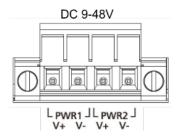
Connect the power jack (in the package) to the UC-4400A Series' DC terminal block (located on the top panel), and then connect the power adapter. It takes about 10 to 30 seconds for the system to boot up. Once the system is ready, the Power LED will light up. All models support dual power inputs for redundancy.
