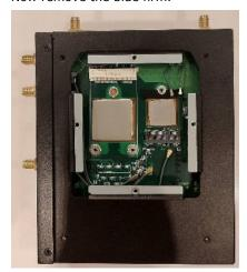
6. Insert the cellular modem into the mPCIe slot. Then, connect the antenna cables to the corresponding modem connectors as shown in the diagram:
