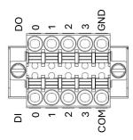
There are four digital inputs and four digital outputs on the top panel. Refer to the figure on the left for detailed pin definitions.
