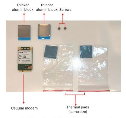
3. Take out the **thinner** alumin block, peel off the blue protective film to expose the adhesive side of the aluminum block, align it with the marked area (red box) on the UC-443xA mainboard and firmly press it into place. The adhesive side should face downward to attach the block securely to the PCB.
