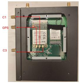
Make sure each connector is securely fastened to ensure signal integrity.
