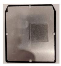
9. Take out the second thermal pad. It has two protective films: one blue and one clear. The clear film covers the adhesive side, which should be attached to the aluminum block. Once attached, remove the blue film to expose the top surface.
