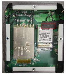
9. Take out the other aluminum block, peel off the blue protective film to expose the adhesive side of the aluminum block, align it with the marked area (red box) on the back of the wireless module door, and firmly press it into place. The adhesive side should face downward to attach the block securely to the module door.
