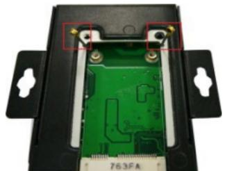
2. Insert the cellular module into the socket and fasten two screws (in the package) on to the top of the module
