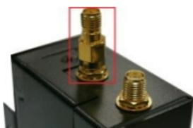
6. Connect the Wi-Fi antennas to the antenna adapters.
