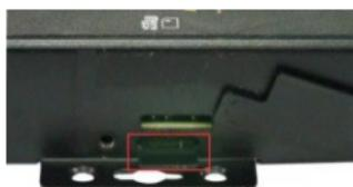
To remove the MicroSD card, simply push the card in and release it.
