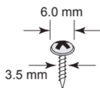
Do not screw the screws in all the way—leave a space of about 2 mm to allow room for sliding the wall mount panel between the wall and the screws.
