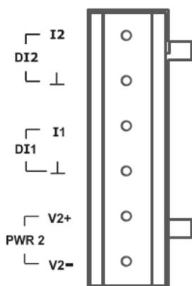
The VPort 451 has four sets of digital input, DI1, DI2, DI3 and DI4. Each DI consists of two contacts of the 10-pin terminal block connector on VPort's top panel. Top and front views of one of the terminal block connectors are shown here.
