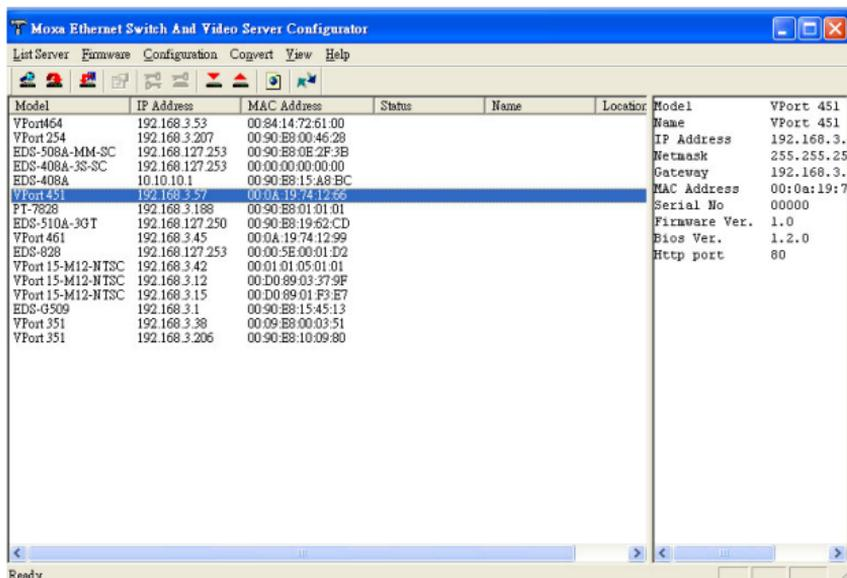
**NOTE** Broadcast Search can only search for devices connected to the same LAN subnet as the VPort. If your devices are located on a different LAN subnet, use the “Specify IP Address” function to search for the device by keying in the IP address.
