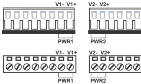
**STEP 1:** Insert the negative/positive DC or AC wires into the V-/V+ terminals.
