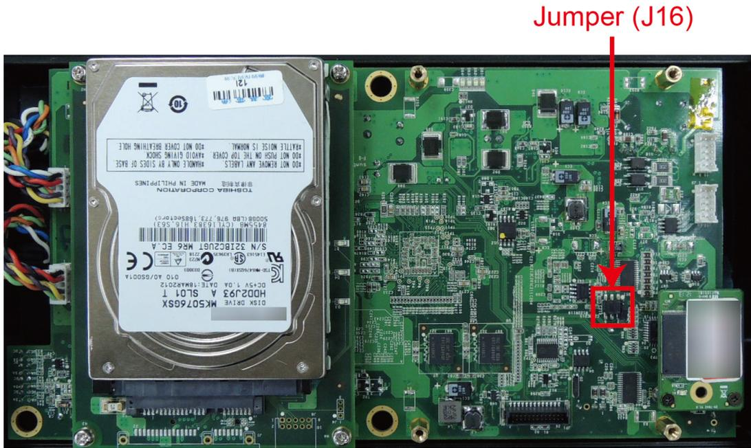
**Step 3:** To switch the IHS mode, adjust the jumpers to one of the configurations shown below.
